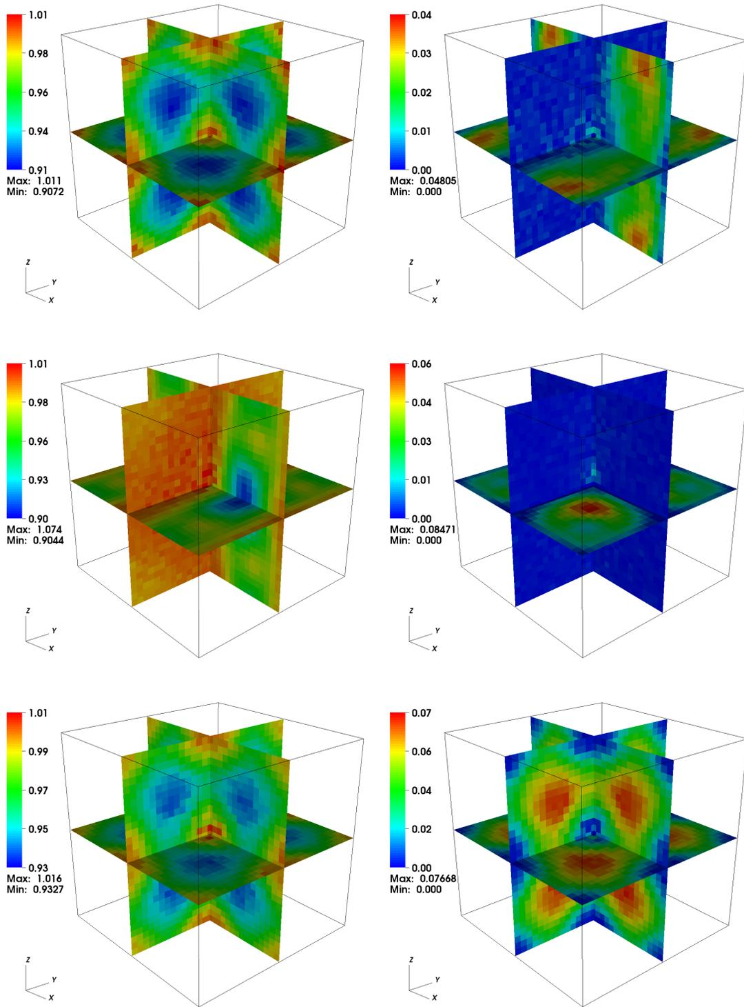
Figure 3: (Left)  $S_{\mathbf{k}}^{(\rho)}$ ,  $S_{\mathbf{k}}^{(v_x)}$  and  $S_{\mathbf{k}}^{(T)}$  (top to bottom); (Right)  $|S_{\mathbf{k}}^{(\rho, v_x)}|$ ,  $|S_{\mathbf{k}}^{(v_x, v_y)}|$  and  $|S_{\mathbf{k}}^{(\rho, T)}|$  (top to bottom) for RK3D-2RNG (Random Direction), with the time step  $\alpha = 0.5$ ,  $\beta = 3\beta_T/2 = 0.1$ , periodic boundary conditions with  $30^3$  cells, and averaging over  $10^6$  time steps.
