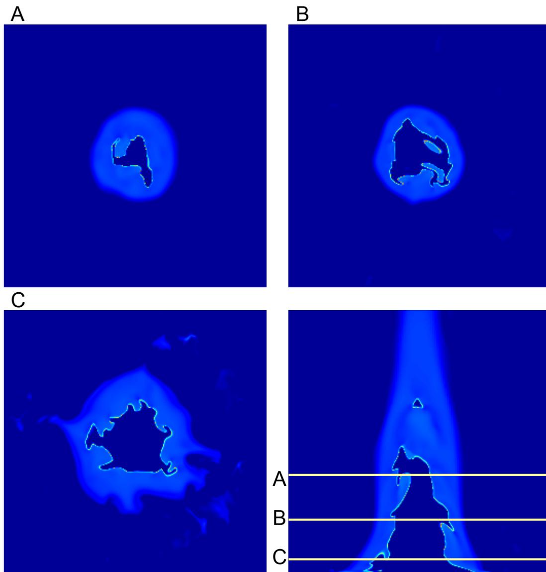
**Figure 3.** Raster images of the CO mole fraction over the computational domain. The lower right image is a vertical slice through the center of the domain. The three labelled images correspond to horizontal slices taken at the corresponding labelled locations in the vertical slice.
