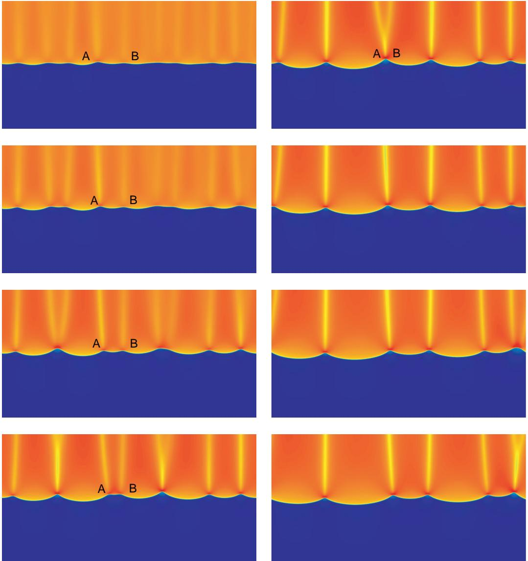
Fig. 3. Time history of LD simulation, showing coalescence of LD peaks (e.g., A and B);  $\rho = 5 \cdot 10^7 \text{ g/cm}^3$  and  $T = 10^7 \text{ K}$ . Shown is vertical flow velocity. The ‘searchlights’ are regions of lower flow speed in the ash (see Figure 4.) Time increases down the left hand column from  $.78 \mu\text{s}$  and continues down the right column to  $3.4 \mu\text{s}$ .
