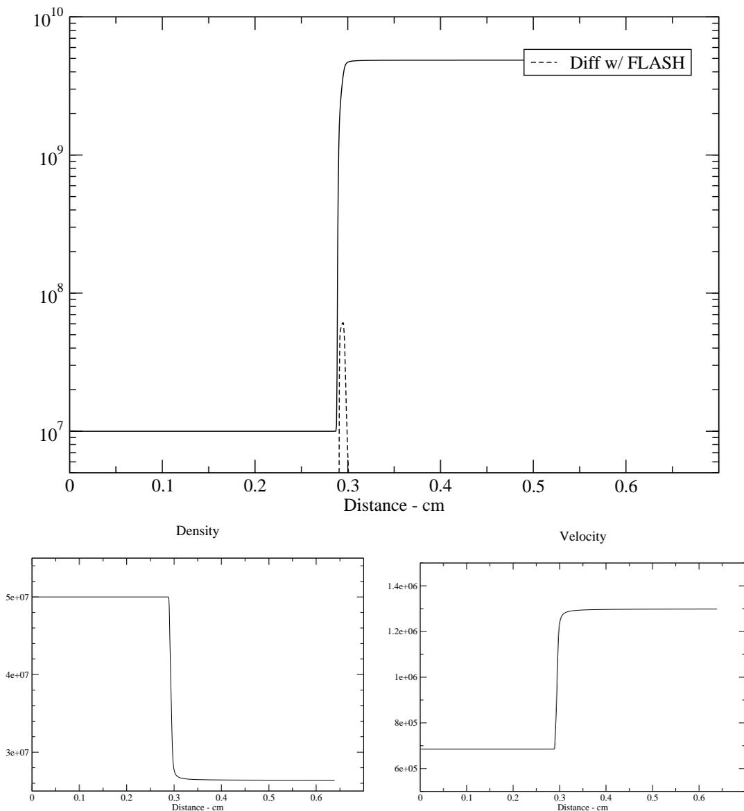
Fig. 1. Laminar flame solution for  $\rho = 5 \cdot 10^7$  g/cm<sup>3</sup>,  $T = 10^7$  K. Shown are the solutions for density, speed, and temperature. The difference with the FLASH results from Dursi et al. [32] is indicated on the temperature result
