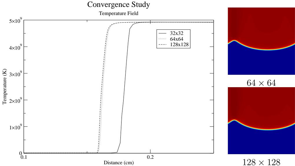
Fig. 2. Two-dimensional convergence study. Left: Curves represent temperature versus distance along a vertical slice through the cusp for base resolutions of  $32 \times 32$ ,  $64 \times 64$ , and  $128 \times 128$ , with 2 levels of refinement  $.420 \mu\text{s}$ . Right: image of temperature field at medium and finest resolutions.
