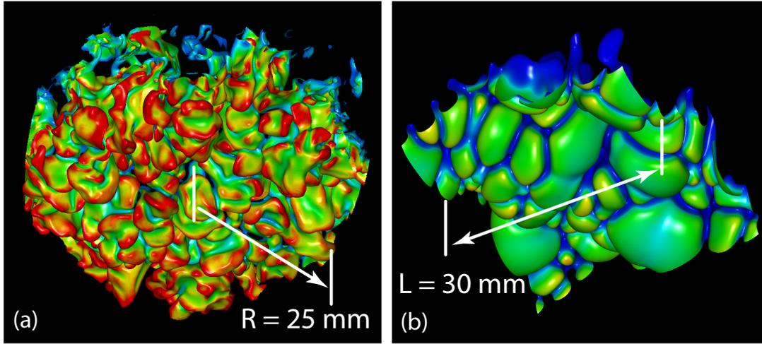
Figure 6: Flame isotherm,  $T = 1144$  K, colored by the local rate of  $H_2$  consumption. (a) Low-swirl flame isotherm, conditioned on  $r < 25\text{mm}$ ,  $z < 8\text{mm}$ . (b) Representative isotherm of an idealized  $\phi=0.37$   $H_2$ -air flame propagating freely in uniform flow.
