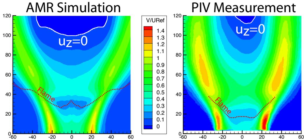
Figure 5: Comparison of the mean vertical velocity (scaled by the mean fueling rate) for the simulated ideal low-swirl nozzle, and a representative experimental profile. A number of key features are recovered in the simulations, including the weak recirculation approximately 10 cm downstream of the nozzle. The computed flame position sits somewhat downstream of the measured data, consistent with the simulation’s higher mean velocity in the core.
