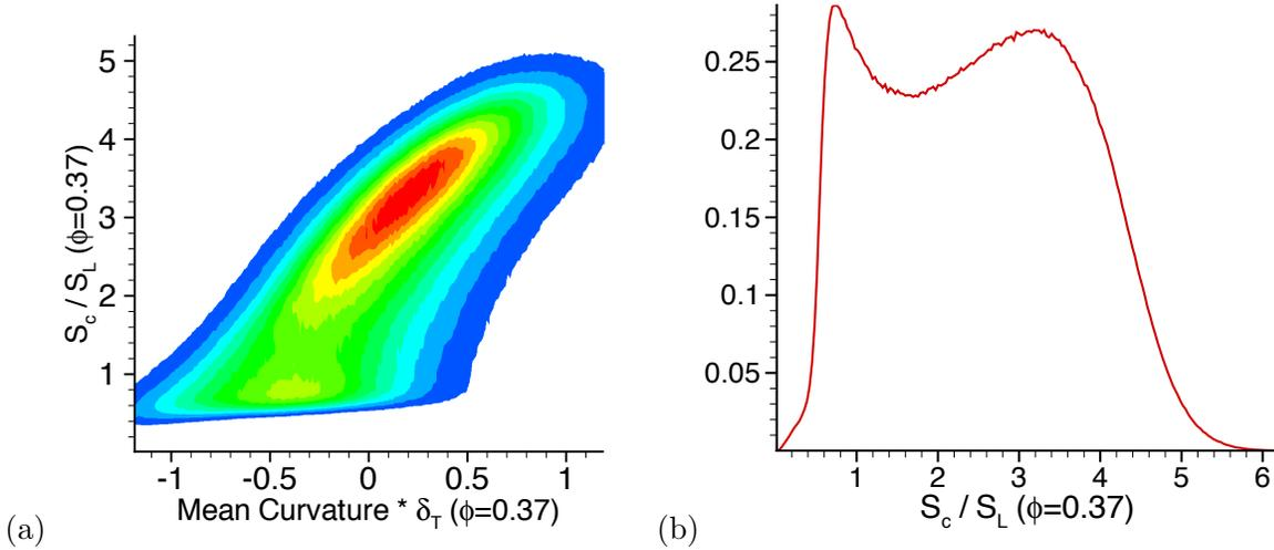
Figure 10: (a) Joint PDF of local consumption speed,  $s_c^\ell$ , with mean curvature, (b) Distributions of  $s_c^\ell$  over the entire conditioned flame surface. In both plots, the burning speed is normalized by the speed of the flat  $H_2$ -air flame at  $\phi=0.37$ .
