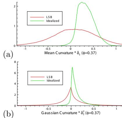
Figure 8: Distributions of mean and Gaussian curvatures of the flame isotherm (conditioned on  $r < 5$  cm,  $z < 8$  cm), scaled to the thermal thickness of the laminar  $H_2$ -air flame at  $\phi=0.37$ .
