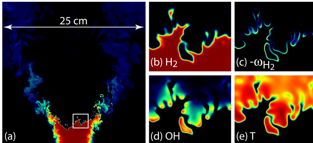
Figure 3: Typical slice from a snapshot in time of the computed flame solution. Panel represents a vertical slice centered on the symmetry axis of the nozzle. (a) The mole fraction of  $H_2$  over a  $(25 \text{ cm})^2$ . (b)-(e) Enlargements of the white-boxed region (approx. 2.5 cm wide) in (a). (b)  $H_2$  mole fraction, (c) Destruction rate of  $H_2$ , (d) Mole fraction of  $OH$ , and (e) temperature. All scales are relative to the peak values over the domain at that instant.
