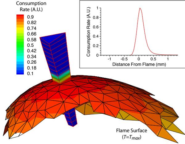
Figure 9: Prism-shaped volume,  $\Omega$ , constructed using curves locally normal to the temperature isotherms (both the flame and  $\Omega$  are colored by a typical profile of fuel consumption rate,  $\omega_{H_2}$ ). The inset plot shows the variation of  $\omega_{H_2}$  normal to the flame surface.  $\Omega$  discretizes the flame volume, and the integral curves of  $T$  that bound  $\Omega$  define a set of local flame coordinates.
