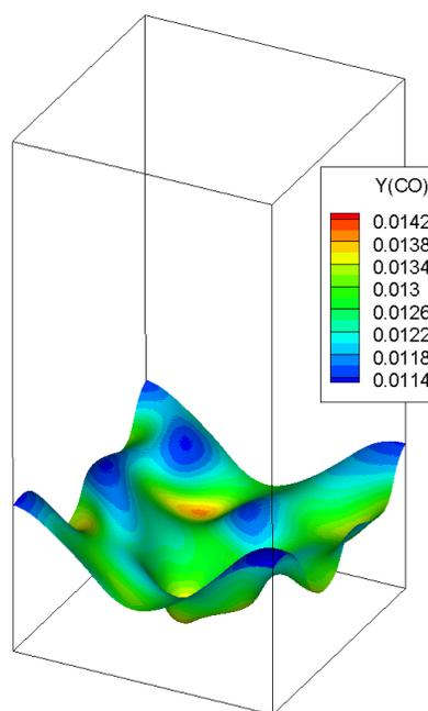
**Figure 2:** Temperature isosurface colored by CO mass fraction.
