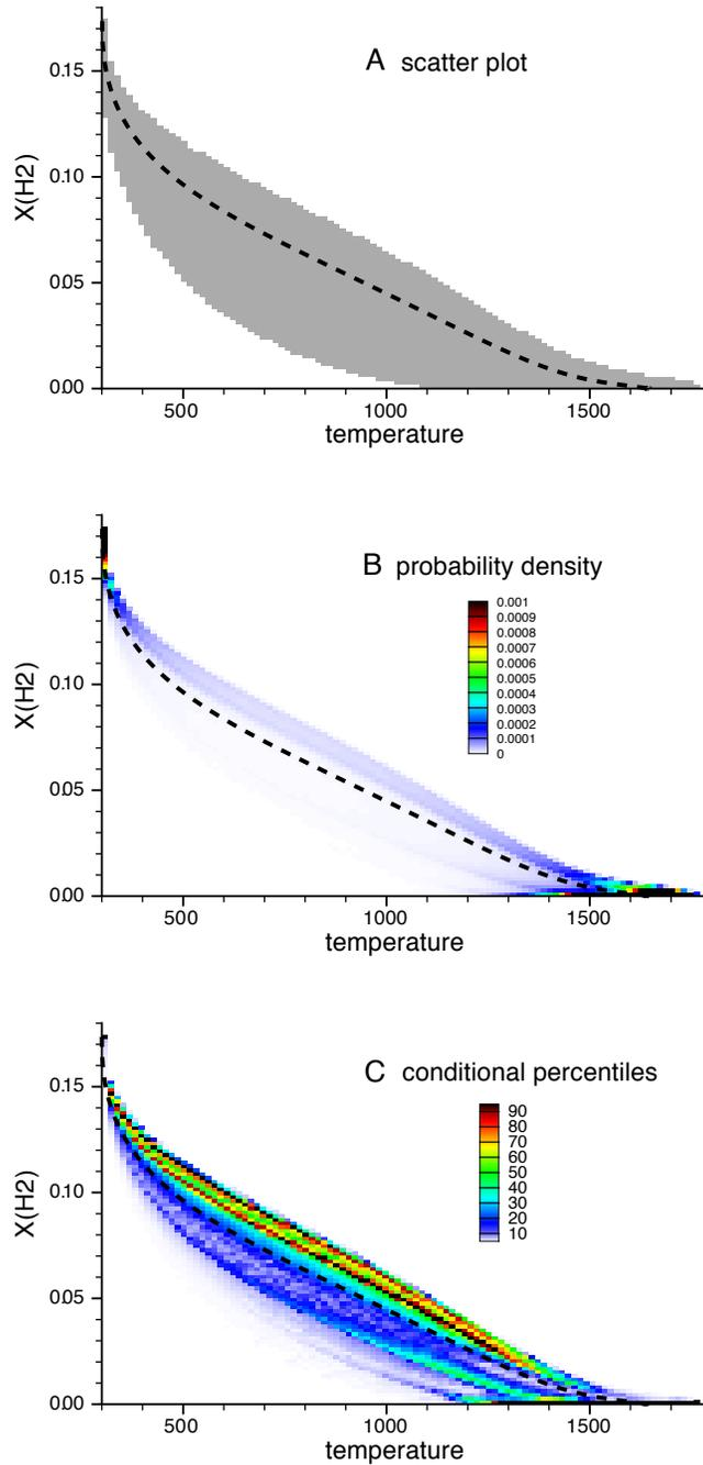
**Figure 2: Joint distribution of fuel and temperature in the premixed hydrogen flame depicted three ways. In each plot the dashed line is the distribution for a flat laminar premixed flame calculated by the CHEMKIN software PREMIX [3].**
