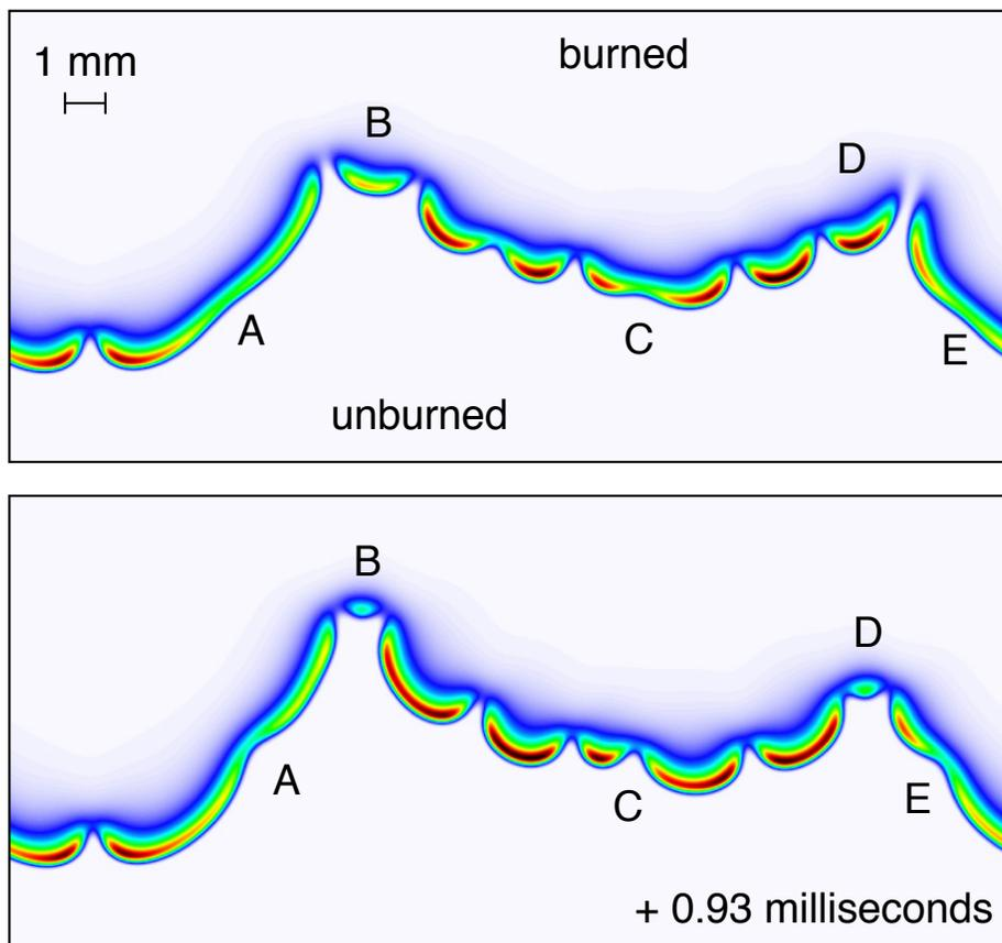
**Figure 1: The freely propagating premixed hydrogen-air flame ( $\phi = 0.5$ ) at two instants in time: earlier (above) and later (below). Pictured is the mole fraction of atomic hydrogen,  $X(\text{H})$ , in a linear rainbow scale from 0.0 (white) to 0.0069 (black).**
