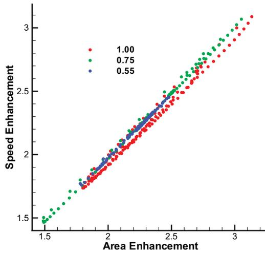
Figure 9: *Turbulent flame speed versus flame area.*
