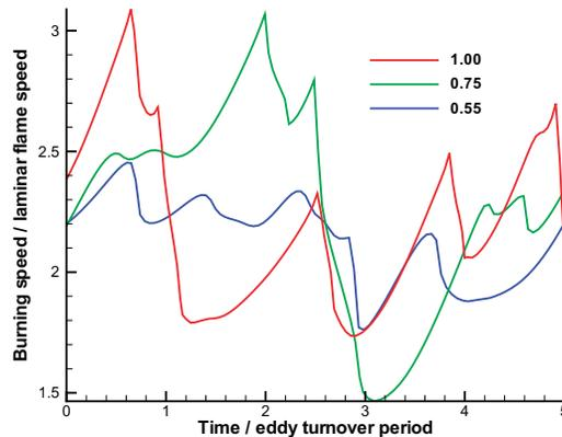
Figure 7: *Turbulent flame speed for the three flames.*
