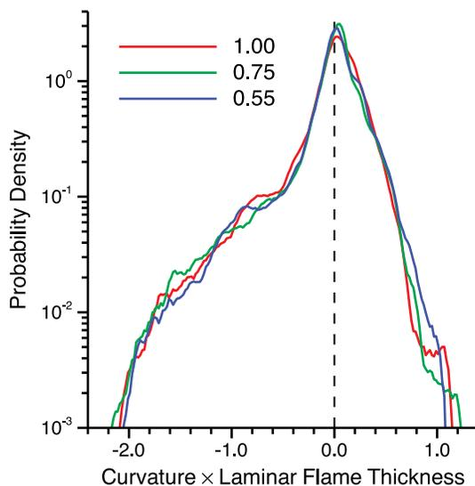
Figure 6: *Probability density of curvature scaled by laminar flame thickness for the three flames of different stoichiometries. Density is calculated by a moving average over 5 intervals of width 0.02 (nondimensional) on the horizontal axis.*
