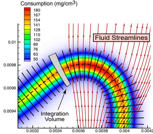
Figure 11: *Construction of local control volumes at a typical flame surface. The volumes are centered on the flame, and extend normal to the local isopleths in progress variable at uniform intervals along the flame. Adjacent flame normals define a volume over which we define the local consumption-based burning speed.*
