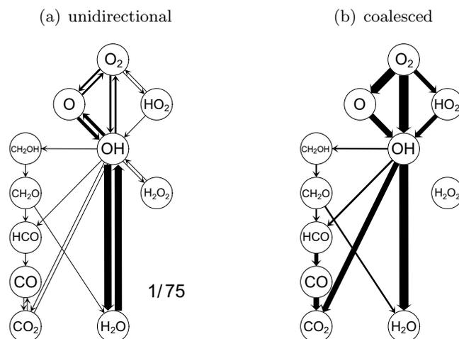
Figure 2: Oxygen reaction path diagrams (a) based on the unidirectional halves of each reversible reaction, and (b) with only the net direction shown. Figure (a) is drawn to  $1/75$  the scale of the other; its thickest path is  $\text{OH} \rightarrow \text{H}_2\text{O}$  at  $1.28\text{e-}02$  (mol/s). The thickest net path in (b) is  $\text{O}_2 \rightarrow \text{OH}$  at  $2.21\text{e-}4$  (mol/s). Only arrows at least 10% of the thickest net path are shown.
