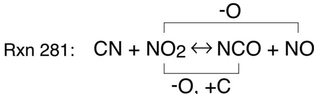
Figure 16: Example of a potentially ambiguous reaction. The CHEMKIN specification does not indicate whether this reaction simply exchanges an O atom from NO<sub>2</sub> to the CN molecule or if it represents a multi-step exchange event.
