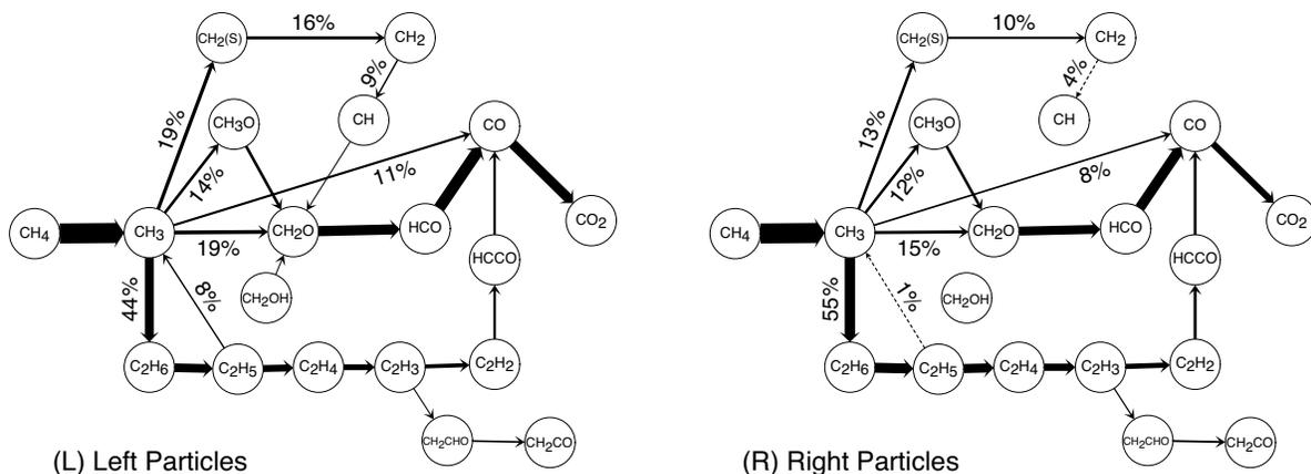
Figure 7: Carbon reaction path diagrams for vortex flame interaction,  $\phi = 1.2$ . Here only paths of strength  $> 5\%$  of the largest path,  $\text{CH}_4 \rightarrow \text{CH}_3$ , are shown. For some paths of interest their weights are shown as a percent of the strongest.
