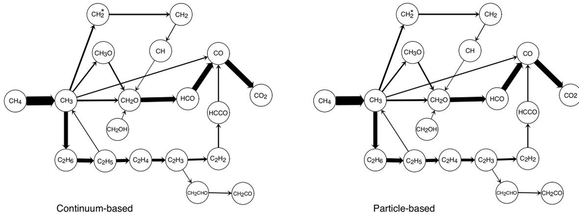
Figure 3: Reaction path diagrams for rich ( $\phi = 1.2$ ) premixed methane flame computed using PREMIX with GRI-Mech 3.0: continuum-based CHEMKIN rate evaluation, and particle-based tabulation of 80,000 trajectories.
