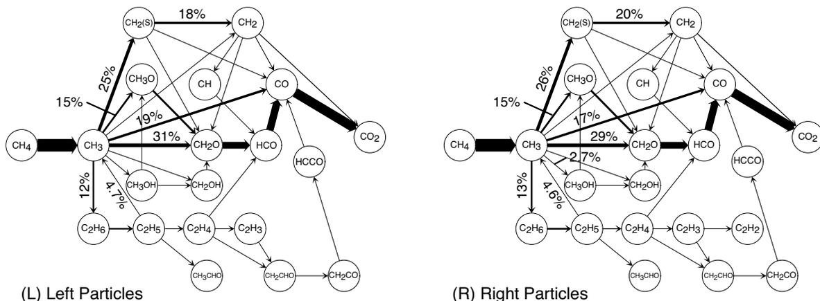
Figure 6: Carbon reaction path diagrams for vortex flame interaction,  $\phi = 0.8$ . Here only paths of strength  $> 1\%$  of the largest path,  $\text{CH}_4 \rightarrow \text{CH}_3$ , are shown. For some paths of interest their weights are shown as a percent of the strongest.
