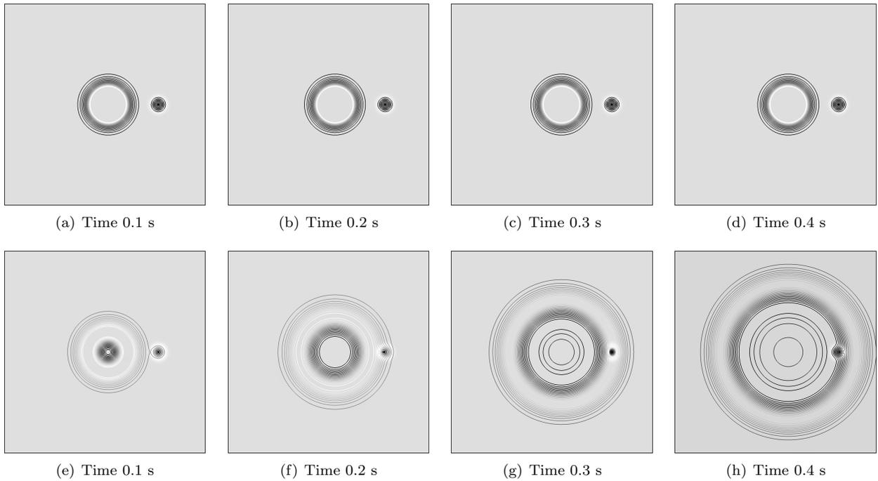
**Figure 1. Isocontour of density superimposed on field of vorticity for solutions at  $t = 0.1$  s,  $0.2$  s,  $0.3$  s and  $0.4$  s. The top row (figures (a)-(d)) are solutions computed with the purely low-Mach-number approach. The bottom row (figures (e)-(h)) are solutions computed with the hybrid method detailed in the present paper.**
