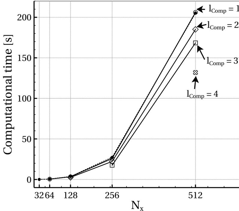
Figure 4. Wall-clock computational time spent to perform simulations with the purely compressible approach (dashed line) and the hybrid method (symbols), and for different maximum level  $L$  of mesh refinement for the low-Mach-number equations. For the hybrid method, circle, diamond, square and cross symbols represent  $l_{Comp}$  set at  $l = 1$ ,  $l = 2$ ,  $l = 3$  and  $l = 4$ , respectively.
