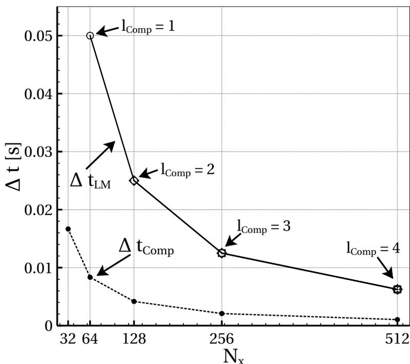
Figure 3. Average time-step employed during simulations performed with the purely compressible approach (dashed line) and the hybrid method (symbols), and for different maximum level  $L$  of mesh refinement for the low-Mach-number equations. For the hybrid method, circle, diamond, square and cross symbols represent  $l_{\text{Comp}}$  set at  $l = 1$ ,  $l = 2$ ,  $l = 3$  and  $l = 4$ , respectively.
